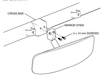
2. Tighten the screws using the tightening torque specified in the Torque Chart.
